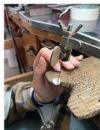
3.b. Jewellery Making: cutting gold disc with handsaw
