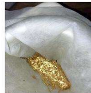
2.c. Extracting Gold: gold residue on filter
